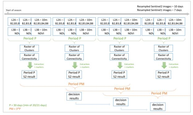
Figure 1-2. Period's representation of the general workflow of the L4D heterogeneity detection algorithm
