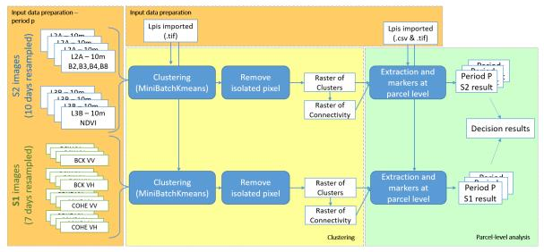
Figure 1-1. General workflow of the L4D heterogeneity detection algorithm
